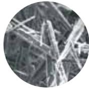
**1) calmat® reduces scale deposits in pipes and appliances.** With the **calmat®** treatment, high-frequency electrical impulses are emitted into the water which changes the crystal formation of the calcium. After the treatment, the adhesiveness of the crystals is reduced so that scale is unable to form in the pipes.
